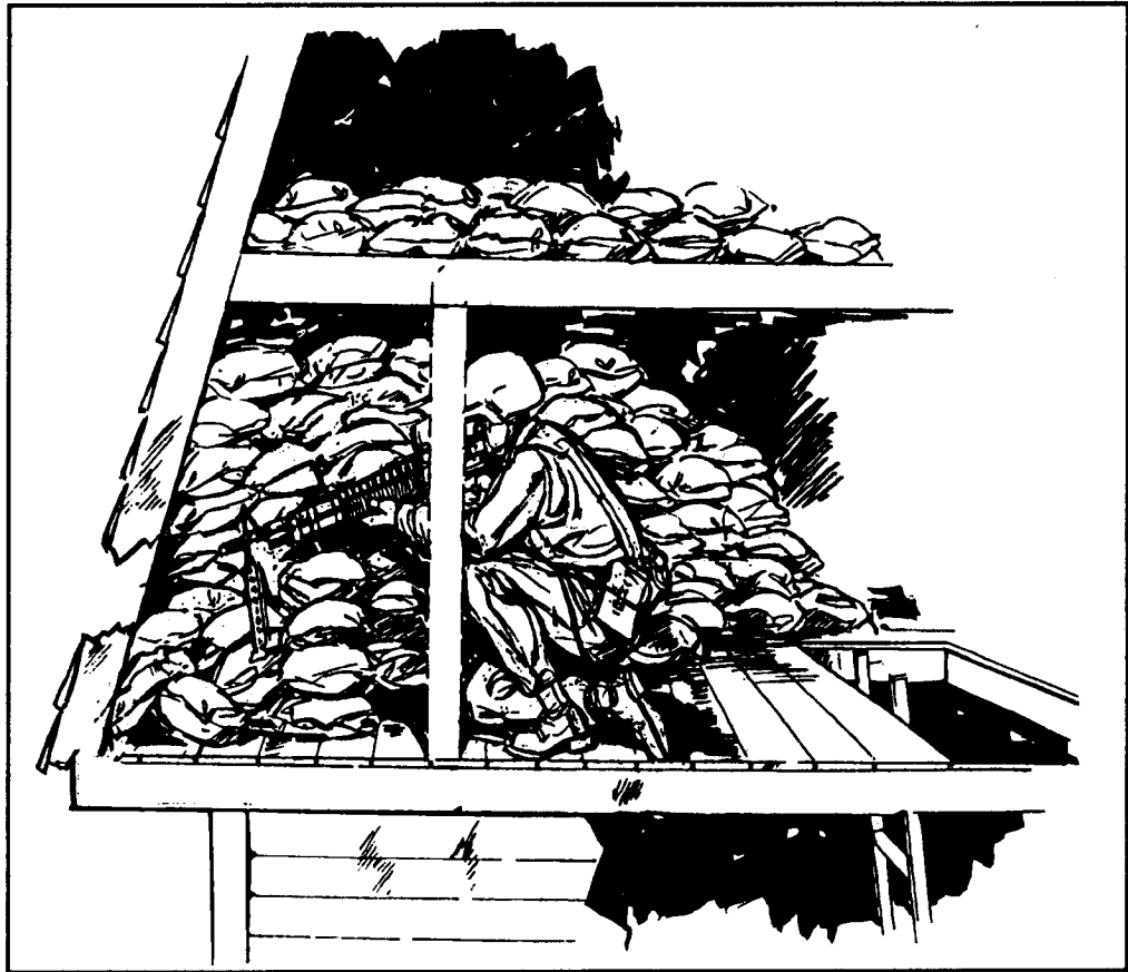
Figure 5-41. Firing platform built under roof.
