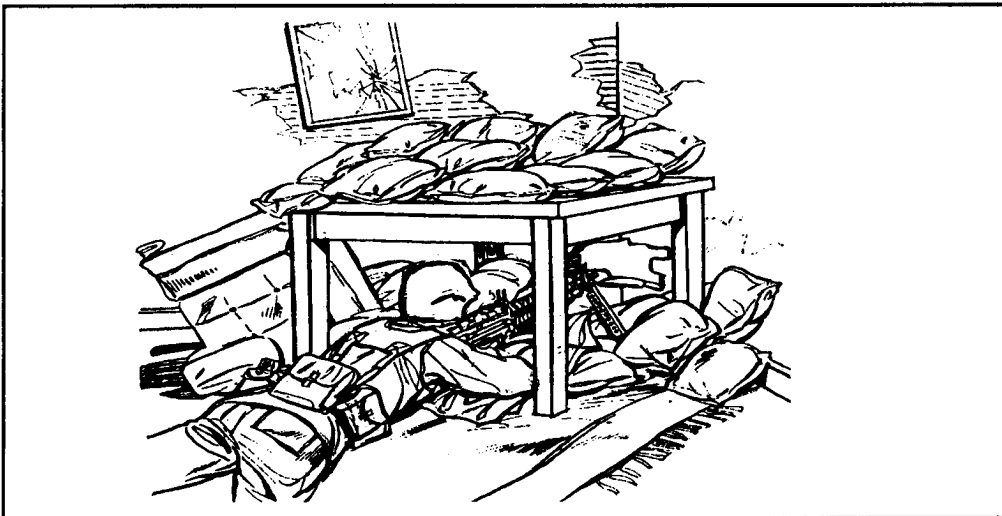
Figure 5-40. Corner machine gun bunker.
